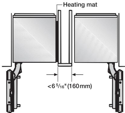
In this case, you will only need the heating mat from the "Merging kit" to avoid condensation and prevent damages. Please be aware the left unit's cutout will require an additional 1/8" (3 mm) to the width to allow installation of the heating mat.
