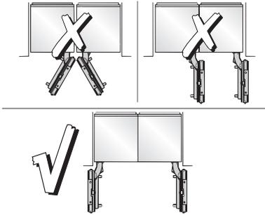
If the appliances are installed directly next to each other (without a partition), they need to be attached together. A heating mat must also be installed. This will help avoid condensation and prevent damages.
